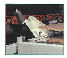
As the panel exits the Adhesive Spreader, it is supported by two rolls, one on either side, mounted at an angle so as not to contact the bottom of the panel. The leading edge contacts and is carried away from the machine, supported by the shuttle.
