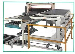
Movement of the laminate rack is controlled by the operator. This moves across the glued board, making the laminate easily accessible to the operator. He pulls off the laminate and positions it on top of the board using edge and end guides to align it with the glued stock.
